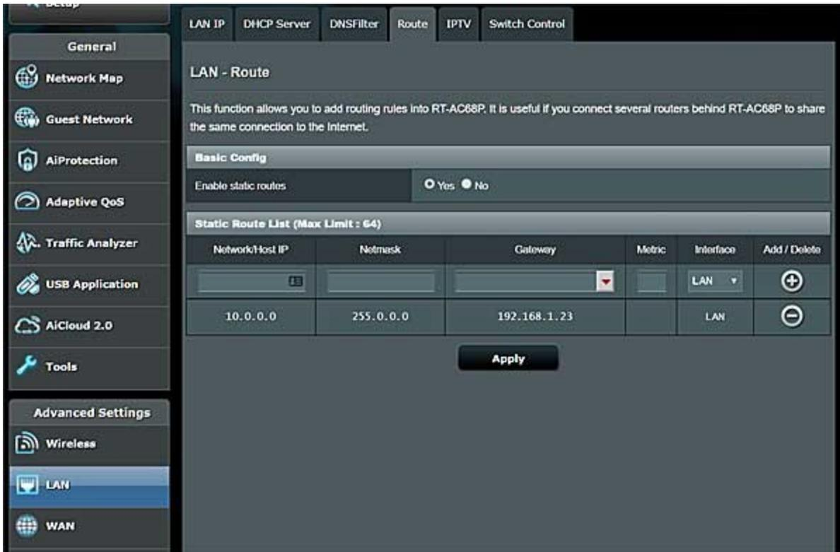
Figure 4 - Asus router static route setup
